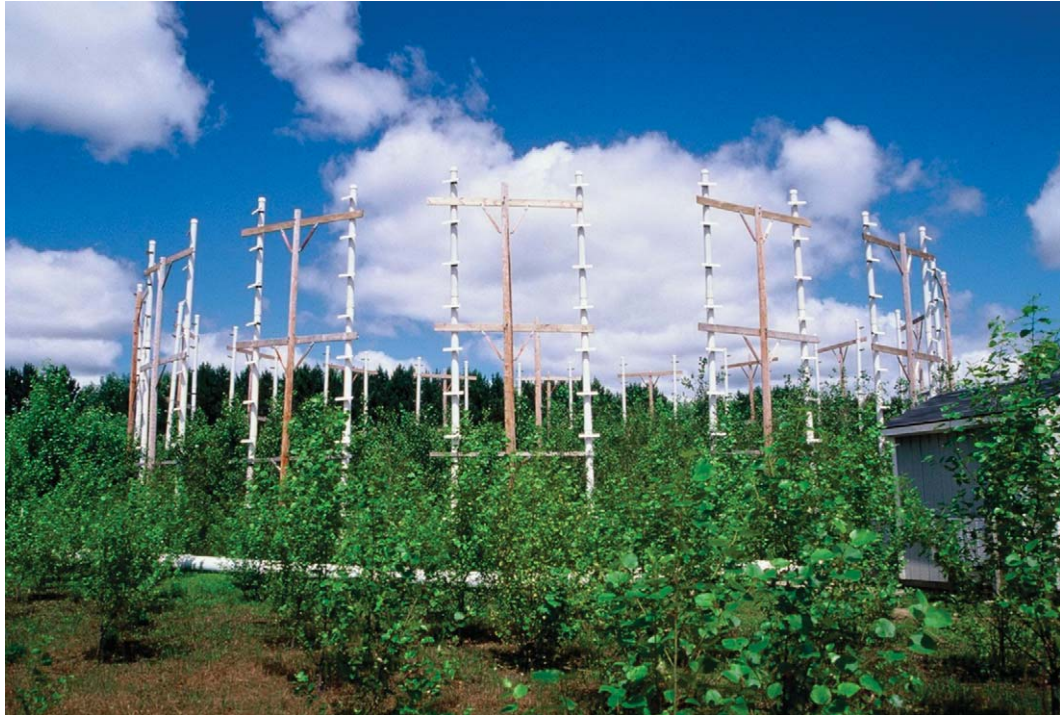
Figure 3 The Aspen FACE (Free Air Carbon Dioxide Enrichment) Experiment is growing trembling aspen trees in the open under carbon dioxide levels similar to those expected to occur late in the twenty-first century. The pipes surrounding the growing trees release carbon dioxide, mimicking the effects of altered atmosphere in a field setting where plants interact with each other and with other environmental variables in a natural setting. Photograph by JP McCarty.
