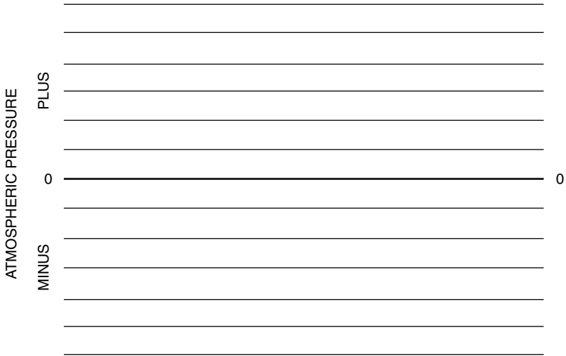
Figure 5.26 Basic plotting grid for pressure gradient diagrams—values typically in inches of water.
