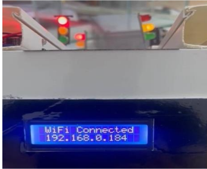
Figure 2: Internet Connection Status Using (16X2) LCD Display
